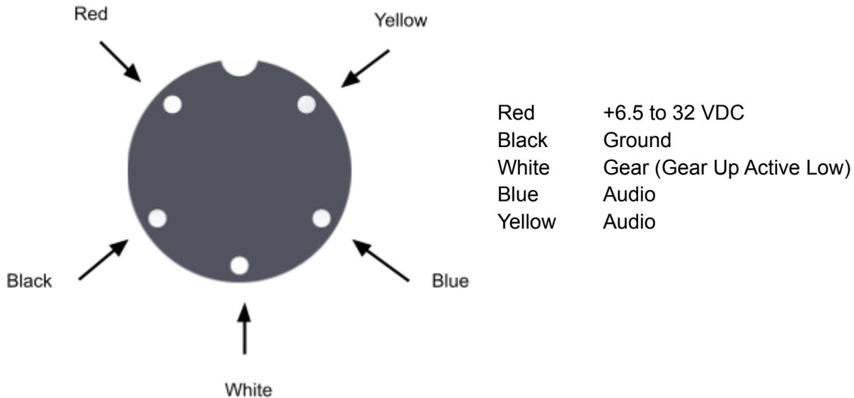
**Reversal of the Power (Red) and Ground (Black) will cause internal damage to the circuitry and is not covered under warranty!**
